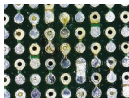
FIG 2: Open via and solder resist damage.
