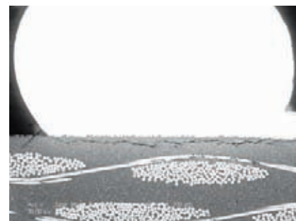
FIG 3: Partial pad crater. (Photo is courtesy of Michael Meilunas, Universal Instruments Corp., Advanced Research in Electronic Assembly (AREA) Consortium)
